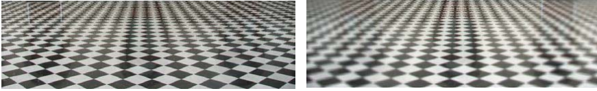
Field curvature aberration produces increasing defocus and loss of contrast away from the field center. (Left) original scene. (Right) simulated image in the presence of field curvature aberration.
