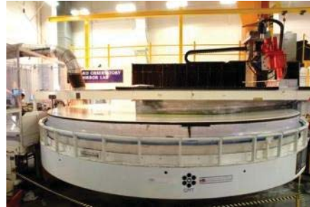
Figure 8. The Large Optics Generator uses diamond tools to cut the surface shape into one of the 8.4-meter diameter off-axis mirror segments for the Giant Magellan Telescope. These mirrors have 14.5 mm deviation from the natural spherical shape.
