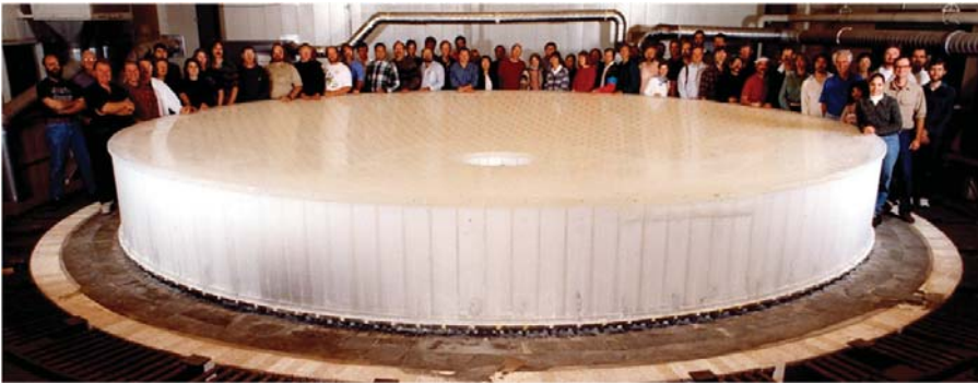
Figure 5. The 8.4-meter diameter LBT primary mirror blank cast of low-expansion borosilicate glass in the spinning furnace at the University of Arizona's Steward Observatory Mirror Lab.
