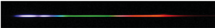
Figure 4. Super-continuum of laser light generated from short pulses sent through a nonlinear micro-structured fiber. A zoomed-in look at this spectrum would reveal a discrete frequency comb structure rather than a continuous distribution of frequencies.
