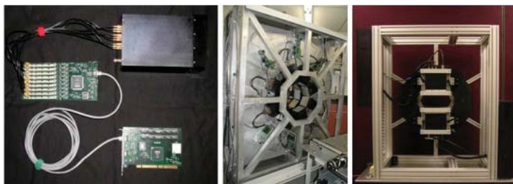
Figure 6. University of Arizona Center for Gamma-Ray Imaging modular gamma camera with list-mode electronics (left). Arrays of cameras are used with collimators to build SPECT systems (center) and with coincidence-timing to build PET systems (right).
