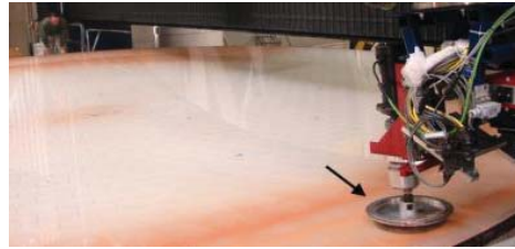
Figure 9. Accurate polishing of the GMT mirrors requires computer-controlled stroking of tools on the surface to wear down the desired regions of the optical surface. The tools are made to fit the aspheric surface by computer control for the stressed lap on the left, and using flow of a viscoelastic compound for the 30 cm tool on the right.
