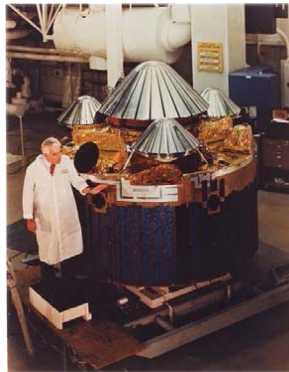
Fig.3. The Pioneer Venus Multi-probe delivery spacecraft. The large cone-shape in the middle is the large probe that carried the Solar Flux Radiometer to the surface of Venus.
