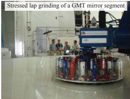
Figure 9. Accurate polishing of the GMT mirrors requires computer-controlled stroking of tools on the surface to wear down the desired regions of the optical surface. The tools are made to fit the aspheric surface by computer control for the stressed lap on the left, and using flow of a viscoelastic compound for the 30 cm tool on the right.
