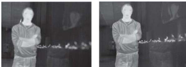
Figure 5. An image from the traditional thermal camera that is blurred due to defocus from close objects such as the person (left). The EDoF computational thermal camera delivers crisp images including close objects (right).
