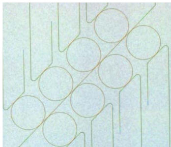
Figure 2. Silicon photonics backbone of a 4 channel EO polymer/silicon reconfigurable optical add drop multiplexer; the rings are about 100 microns in diameter.
