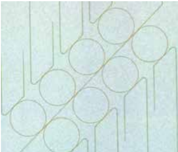
Silicon photonic microring resonators for ultracompact high-speed optical switching. (Image courtesy of Norwood lab)
