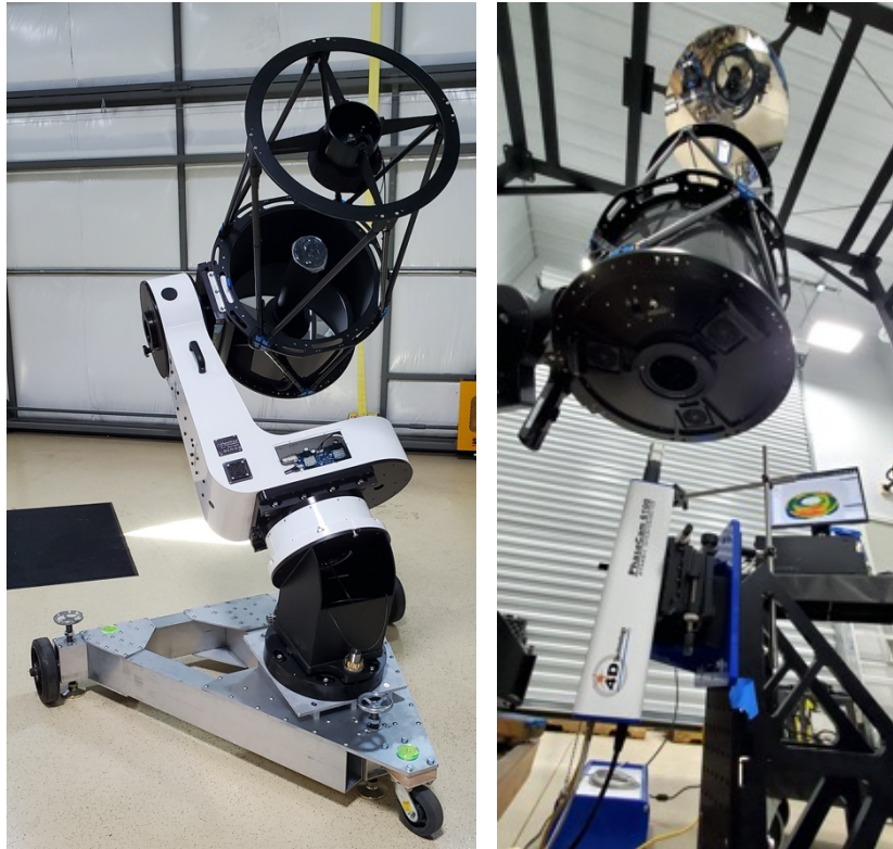
Figure 5. (Left) My new 20-inch Planewave CDK telescope in my shop in Oregon on a homemade roll-out base for initial testing. The base wedge is set for the latitude of the observatory in Chile so there's an additional compensator wedge to allow polar alignment in Oregon. The whole assembly weighs about 700 lbs. (Right) The telescope being tested at the factory in double pass against a 45-inch precision Zerodur flat with a PhaseCam 6100 Dynamic interferometer.
