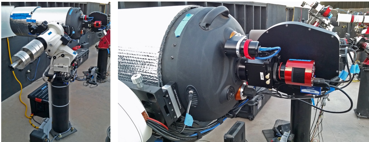
Figure 3. My custom Edge 14 HD at the Deep-Sky West Observatory in northern New Mexico. The image on the left shows the Astro-Physics 1600 German equatorial mount. The telescope itself is wrapped in Reflectix to minimize differential radiative cooling. The image on the right shows the camera, focusing, and guiding instruments. The main CCD imaging camera is out of view behind the large filter wheel holder seen behind the red CMOS guide camera. Small fans behind the primary mirror gently circulate air to prevent laminar thermal air currents inside the telescope tube.
