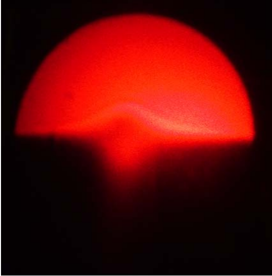
Foucault Test –Near paraxial focus
