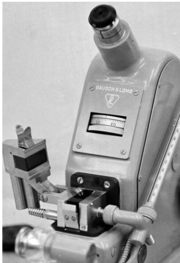
Fig. 2-7. Typical classical Abbe refractometer opened to show prism system.
