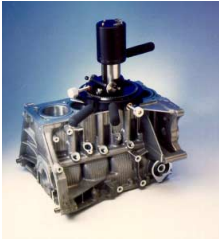
Insight 2000 measuring inside of engine bore
