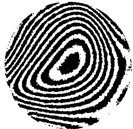
Fig. 5. The measured inhomogeneity of the SFL57 window with the transmission method where the window was rotated 30 deg. The interval of the isometric contour is 0.07 wave, p-v = 0.725 wave, and rms = 0.164 wave.
