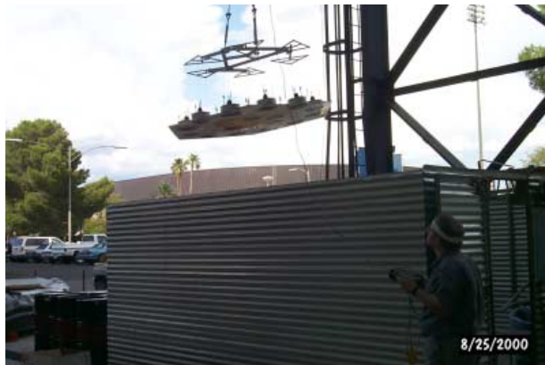
Figure 11. The deblocked facesheet was lifted from the oil bath with an overhead crane.
