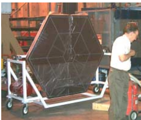
Figure 16. Vacuum support tool and handling cart
