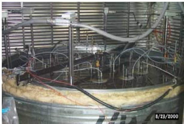
Figure 9. The blocking body with attached facesheet is submerged in a heated oil bath. The floats, which are attached to the facesheet are visible near the surface.
