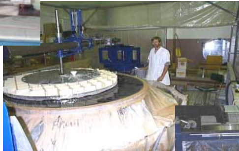
Generate to 3 mm, grind and polish
