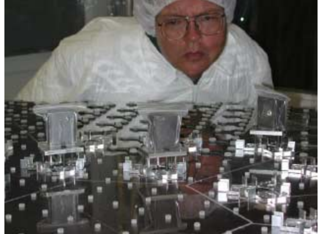
Figure 19. NMSD glass with pucks, some sub-loadspreaders, and gluing jigs.
