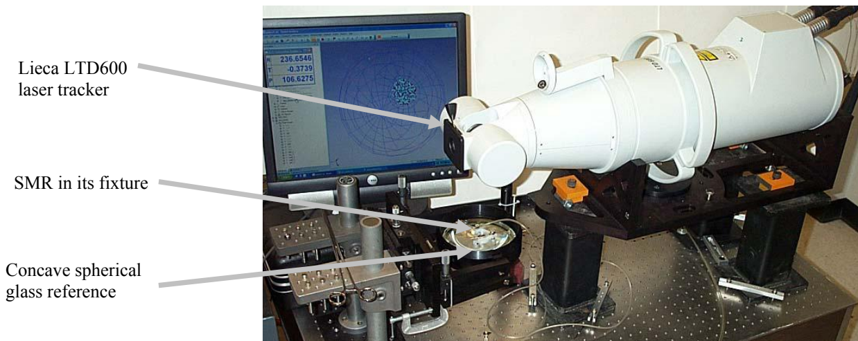
Figure 5. Experimental setup with a Leica LTD600 mounted above the test mirror. The mirror is upward facing and the SMR is mounted in a small vacuum fixture designed to hold the SMR firmly against the mirror surface during data collection. Hemostats are used to reposition the SMR between measurements to avoid thermal effects caused by the operator. Each data point is an average of 50 measurements.
