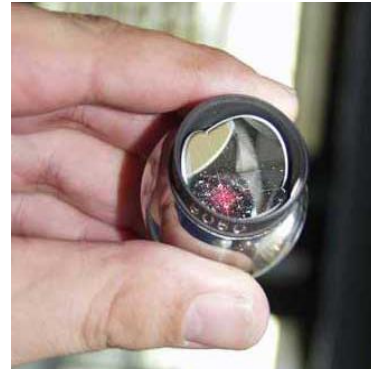
Figure 2. The laser tracker view reflections from SMRs (Sphere Mounted Retroreflectors) or “tracker balls”. These provide an optical reference for the laser tracker and provide a mechanical interface. The tracker measures the location of the center of curvature of the SMR.
