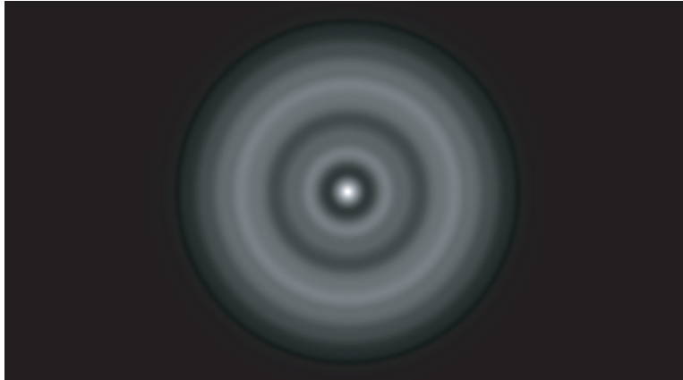
Fig. 5.32. Geometrical estimation of the diffraction pattern from an observation point with N_f = 5 .
