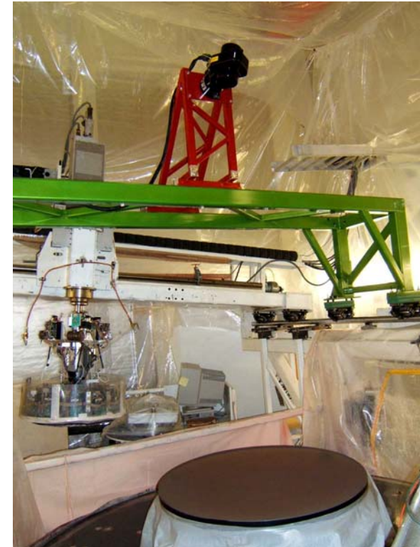
Laser tracker mounted over a 0.95 m mirror. The same arrangement was used for the 1.7 m NST mirror shown to the left.
