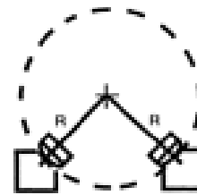
small spherical buttons of a large spherical radius and split Vee Block
