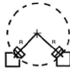
small spherical buttons of a large spherical radius and split Vee Block
