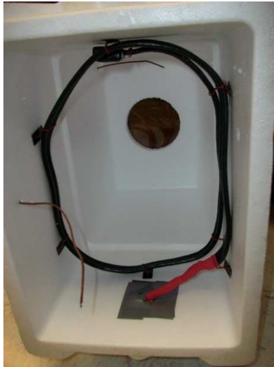
Inside of chamber showing coiled heating wire
