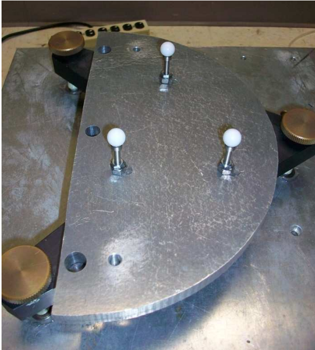
Figure 17: Mounting plate with isolation posts
