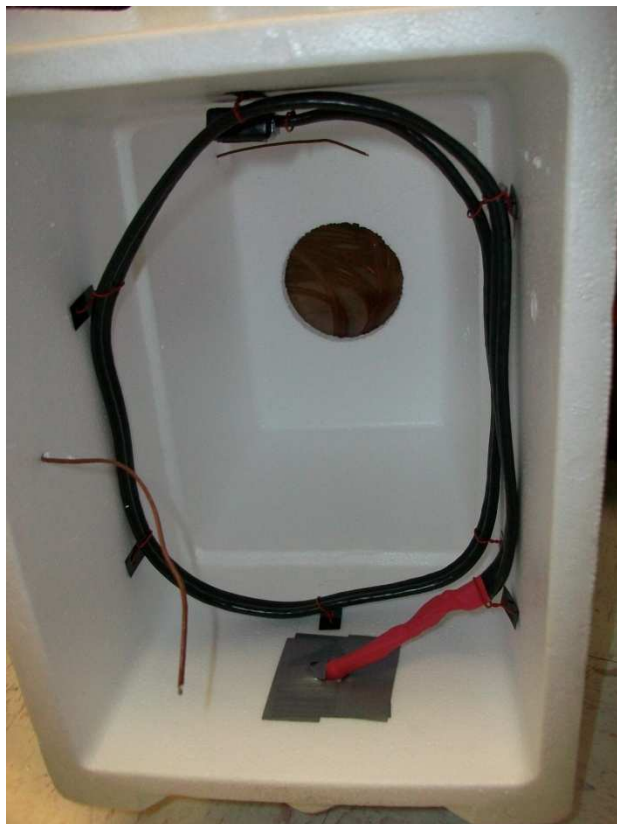
Figure 26: Inside of thermal chamber showing heating element
