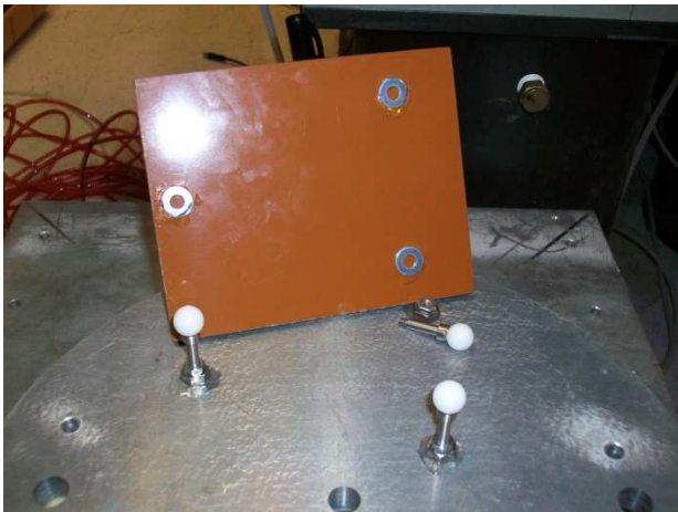
Figure 20: Thermal chamber platform and mounting plate showing stainless steel posts and plastic isolation balls
