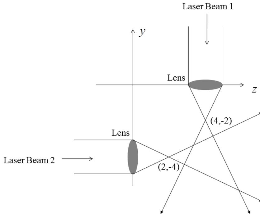
Hypothetical Laser Beam 1 and Laser Beam 2 are coherent and of equal phase and equal amplitude. Each beam is focused by a lens. Locations of foci are shown (units of wavelength). Polarization is out of the plane of the drawing. Ignore diffraction effects.
