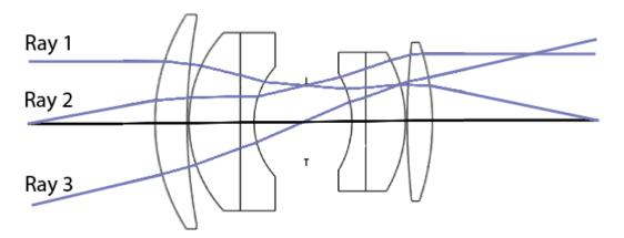
(b) On the figure above, draw the front and rear principal planes and label them P and P', respectively. Label the front and rear nodal points N and N', as well.
