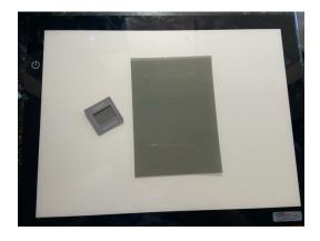
First, affix your first polarizing sheet onto your light source—this will generate linearly polarized light! To reveal the rainbow pattern, look through your second sheet of polarizer at your sample. Try rotating the sample or the second filter. What changes?
