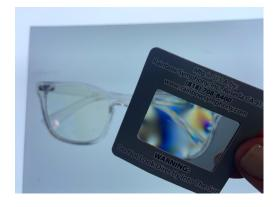
Birefringence depends on wavelength, material thickness and pressure, causing crazy polarization patterns as light passes through them. However, these cool patterns are invisible to the naked eye, so we have to build a simple instrument called a polariscope to reveal them.
