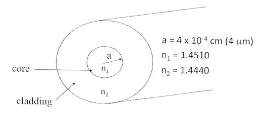
The fiber is made of fused silica, with the cladding pure fused silica and the core doped with germanium ions in order to achieve the elevated refractive index required. The refractive indices are given at 1.550 microns (1550nm), the wavelength at which light is propagated.
