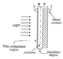
The figure above shows a silicon photodiode. The thin undepleted region is made of silicon also. The refractive index of silicon can be taken as n = 3.4 and the bandgap is  $E_g = 1.1$  eV. All parts are equally weighted.
