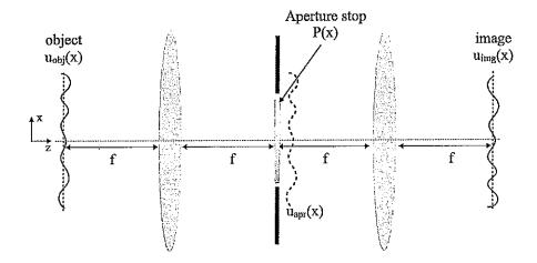
The object and image fields are specified by  $u_{obj}(x)$  and  $u_{img}(x)$  respectively. The front and back focal lengths of the two identical lenses are f = 5cm. In this system you may assume each lens is ideal, that is the lens has no aberrations and it is of infinite extent, so you can ignore any diffraction from the lens itself.
