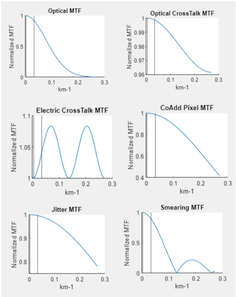
Figure 4: Components of the Overall MTF. The left vertical line on each graph corresponds to visibility for 300km waves and the rightmost vertical line corresponds to visibility for 30km waves.
