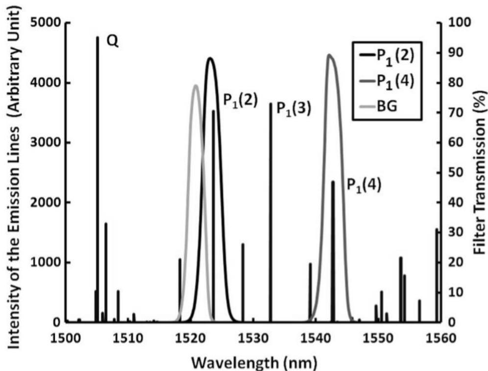
Figure 1: OH (3,1) Band. The gaussian lines are the filter's transmission
