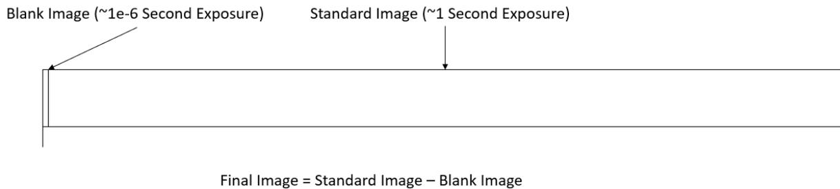
Figure 2: Correlated Double Sampling takes a blank image, which has some noise, and subtracts it from the 1 standard image.
