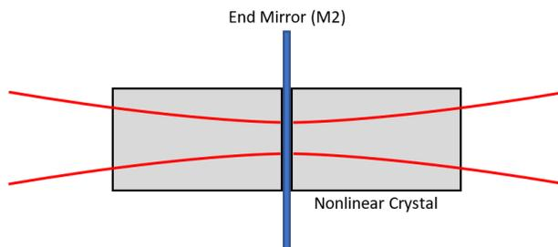
Figure 4. V-cavity unfolded about the end mirror (M2) to demonstrate the double pass through the nonlinear crystal, with the Gaussian beam waist located at the “center” of the crystal.
