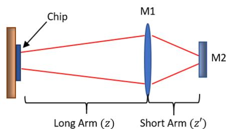
Figure 3. Geometrical representation of unfolded V-cavity. Fold mirror M1 is now represented by a thin lens with similar optical power.
