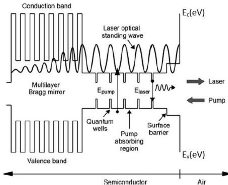
Figure 2. VECSEL semiconductor chip structure. Source: Semiconductor Disk Lasers by Oleg G. Okhotnikov.
