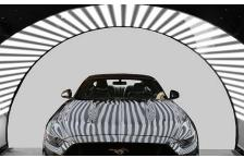
So-called "structured light" systems are critical in industrial inspection, e.g., to detect defects in car bodies [2]
