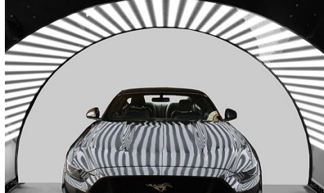
So-called “structured light” systems are critical in industrial inspection, e.g., to detect defects in car bodies [2]
