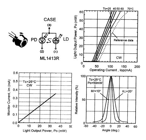
The above data describe the properties of a high power AlGaInP laser with integrated photodiode. The peak emission wavelength is 685nm.
